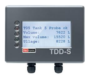
The Truck Driver Display is mounted behind a window pane so that it can be read from the outside. It is attached with Velcro strips. The TDD-S is activated and the illumination is switched on via a motion sensor, which even works through thick, metalised shop windows. The tank content data is automatically transmitted by the Mineo 2 Controller.
