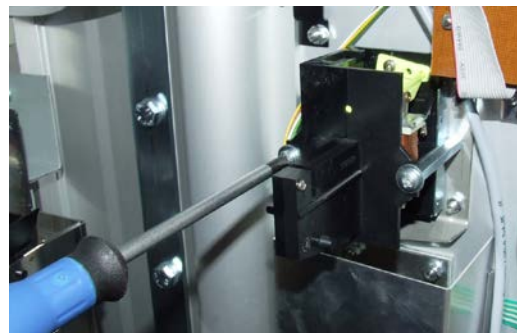
Tighten the screws lightly
